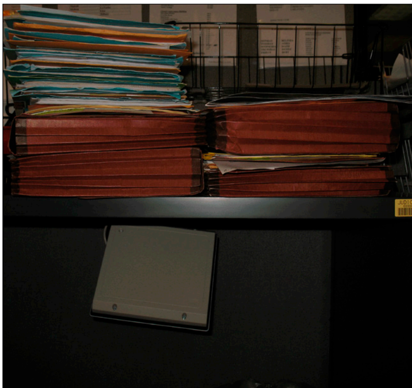
The SmartPad reads multiple tagged files at once, making check-in and check-out much faster.
