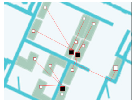
RFID SmartSensors automatically check out files as they arrive at each desk.
